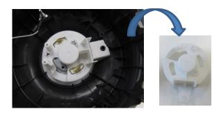
**Step 4:** Remove 4 fixing screws, then you can get out the motor.
