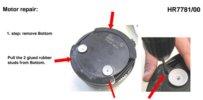
open screws (6x) with a philips screw driver.
