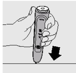
3. Hold the handle upside down and push down on the shaft to release the internal components of the handle.
