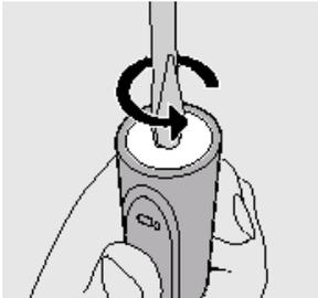
2. Insert a screwdriver into the slot located at the bottom of the handle and turn counterclockwise to release the bottom cap.
