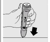
**3.** Hold the handle upside down and push down on the shaft to release the internal components of the handle.
