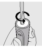
**2.** Insert a screwdriver into the slot located at the bottom of the handle and turn counterclockwise to release the bottom cap.
