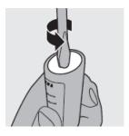
2. Insert a screwdriver into the slot located at the bottom of the handle and turn counterclockwise to release the bottom cap.
