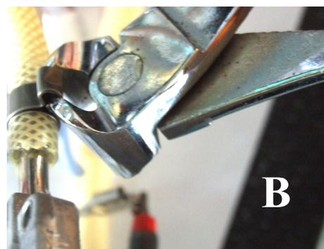
Use a pincers as shown in (B) to remove the clamp
