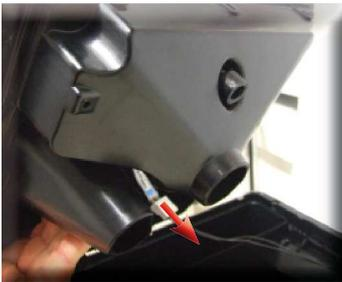
Remove the connection as shown (connection to the cup heater board)
