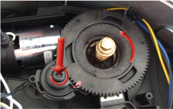
Press down on the grinder adjuster and turn the upper grinder blade support anti-clockwise until it stops.
