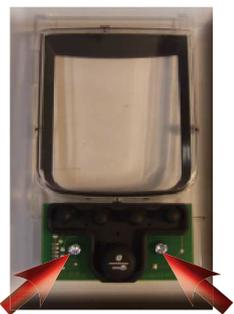
Loosen the screws as shown to remove the KBD MENU board
