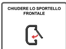
The front door must be closed for the machine to be functional
