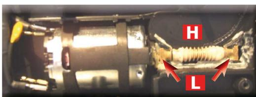
When re-mounting the motor and the transmission shaft, make sure the guides (L) are inserted in the correct housing. Grease the shaft thoroughly and evenly.
