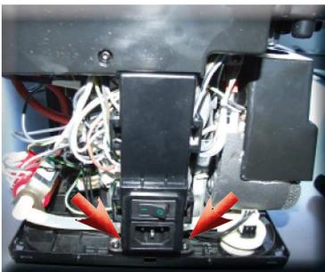
Remove the screws as shown and the component support
