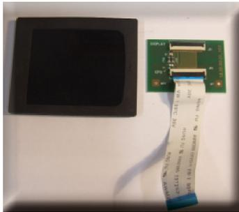
Remove the Display board by unhooking it from the support
