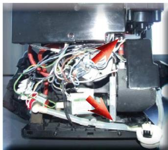
Loosen the screws as shown, remove the boiler assembly support and the electrical and water connections
