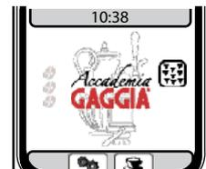
The machine requires a descaling cycle. Damages caused due to the descaling cycle not being implemented non are not covered by the warranty.
