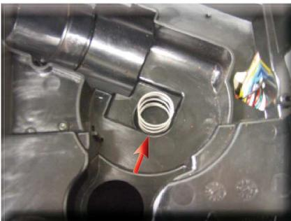
When reassembling the coffee grinder, make sure the spring is repositioned correctly (see picture)
