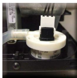
Lift the flow-meter from the component support and remove the electrical and water connections
