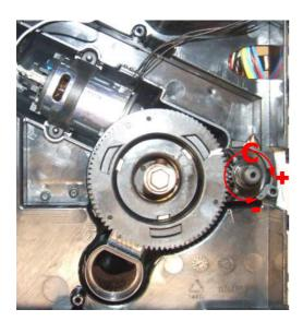
To further adjust the grinding machine, the technician can operate directly on the machine by pressing and turning the highlighted ring nut (C) (clockwise + to increase the grain size and anti-clockwise - to decrease it)
