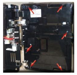
Loosen the screws as shown to remove Loosen the screws as shown the inner cover of the front panel
