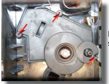
Loosen the screws as shown and remove the sound insulating cover of the coffee grinder
