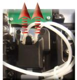
Remove the Teflon pipe support assembly
