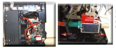
Remove the two pump supports (highlighted) anchored to the structure and disconnect the electrical and water connections
