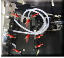
Loosen the screws shown and remove the front panel insert
