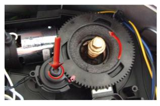
Press down on the grinder adjuster and turn the upper grinder blade support anti-clockwise until it stops.
