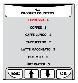
The number of dispensing cycles performed by the machine is displayed for each product. The counters cannot be reset. The value may be different from that shown in the user menu as the latter can be reset. Press ESC to return to the main menu.
