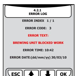
A maximum of 20 errors may be saved and displayed (when the 21st error occurs, the system saves it by deleting the first error read).
