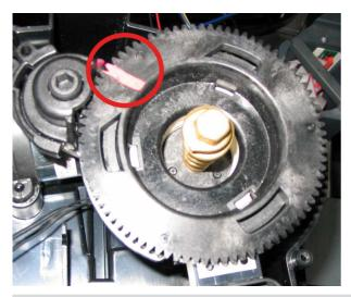
The two notches must overlap in order to adjust the base.
