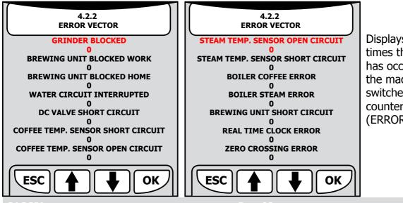
Displays the number of times that a given error has occurred, from when the machine was first switched on or when the counters were last reset (ERROR RESET function).
