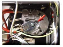
Loosen the screw as shown and remove the electrical and water connections
