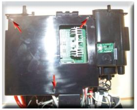
**1**)Loosen the screws as shown and remove the board cover
