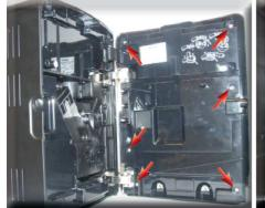
Loosen the screws as shown to remove the inner cover of the front panel
