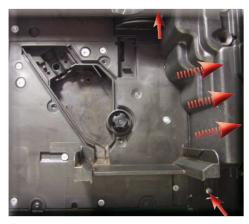
Loosen the screws as shown and remove the frothing valve protection
