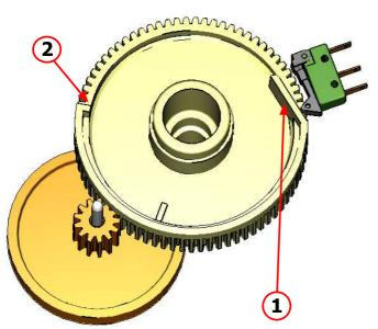
The gearmotor is activated by a direct current motor that acts on the smaller double toothed wheel via a worm screw. The unit is mounted on the axle of the large toothed wheel and when a coffee is requested, it moves from the idle position to the dispensing position to then return to the idle position.
