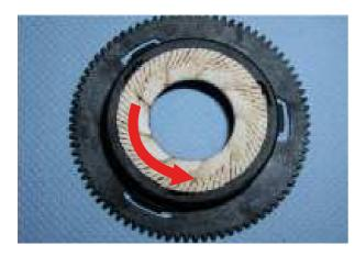
Turn the grinder blades clockwise from the support. The bayonet fittings can be accessed from the rear.
