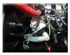
Remove the two pump supports (highlighted) anchored to the component support and disconnect the electrical and water connections
