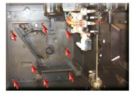
Loosen the screws as shown and remove the gearmotor cover
