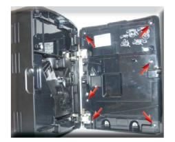
Loosen the screws as shown to remove the inner cover of the front panel
