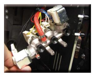
Disconnect the electrical and water connections
