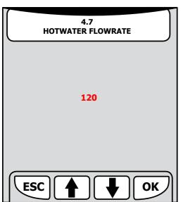
Indicates the capacity (in litres/hour) of the hot water / steam circuit pump. Press "OK" to edit the setting.
