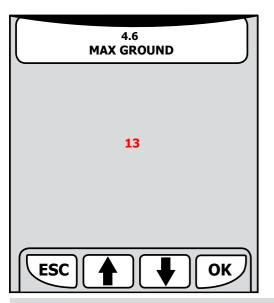
Indicates the maximum number of coffee dregs in the dreg container. Press "OK" to edit the setting. The default value is 13.
