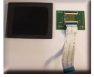
Remove the Display board by unhooking it from the support
