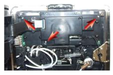
Loosen the screws as shown and remove the CPU board
