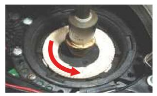
Turn the grinder blades anticlockwise from the support.
