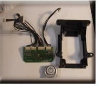
Loosen the screws as shown to remove the KBD STAND-BY board
