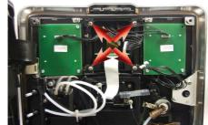
Remove the connections, loosen the screws as shown and remove the front panel
