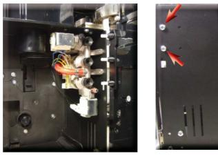
Loosen the screws as shown, making sure that the frothing valve does not fall and damage the connections
