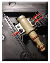
Loosen the screws as shown and remove the boiler pin
