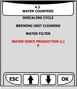
**WATER SINCE PRODUCTION**: indicates the number of litres of water used since the machine was first switched on
