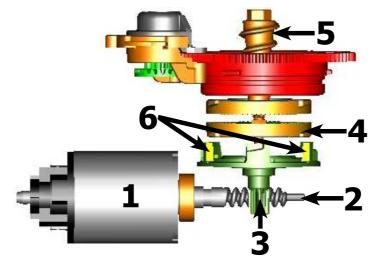
The coffee grinder is activated by a direct current motor (1) via helicoidal wheel transmission and a worm screw (2).
